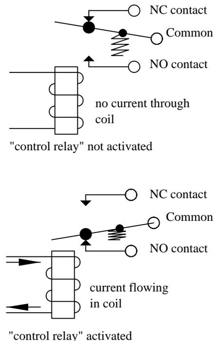
Figure LC-2: Control relay with NO and NC contacts
