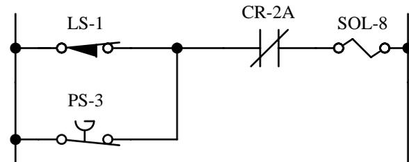
$$\text{SOL-8} = ((\text{not LS-1}) \text{ or } (\text{not PS-3})) \text{ and } (\text{not CR-2A})$$
