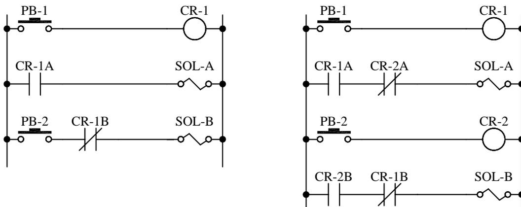
Figure LC-8: Prevention of simultaneous coil energizing
