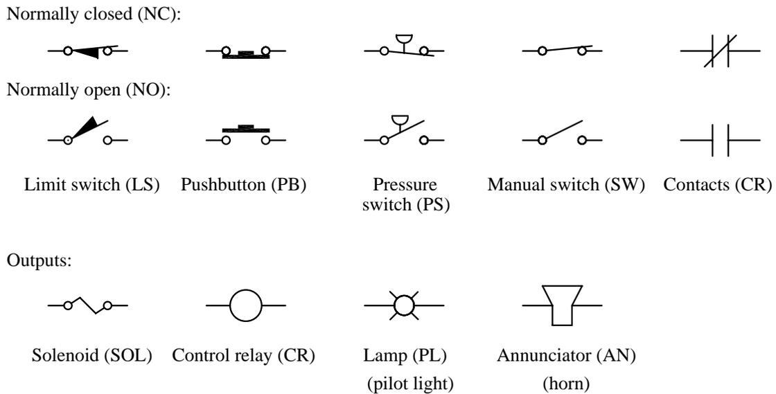
Figure LC-3: Ladder logic schematic elements
