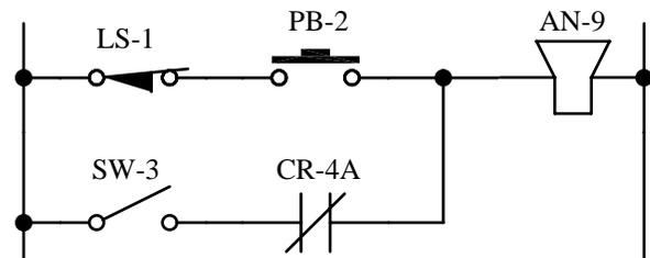
$$\text{AN-9} = ((\text{not LS-1}) \text{ and } \text{PB-2}) \text{ or } (\text{SW-3} \text{ and } (\text{not CR-4A}))$$
