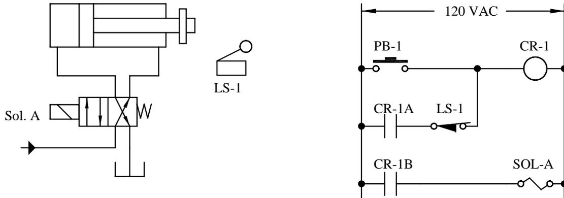
Figure LC-1: Simple pneumatic and logic control system
