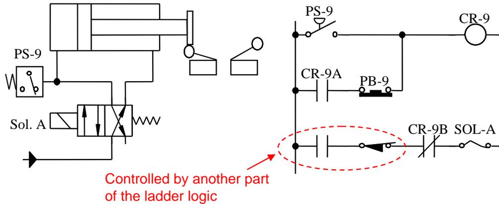
Figure LC-7: Cylinder "jamming" protection
