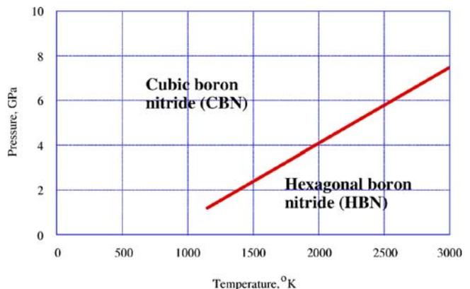
**Fig. 2** The equilibrium phase diagram of hexagonal boron nitride and cubic boron nitride [6]
