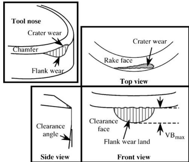
Fig. 3 Typical wear patterns on a finishing tool [14]
