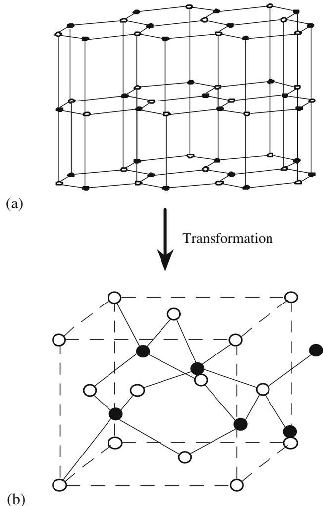
**Fig. 1** The arrangement of atoms in boron nitride: **a** hexagonal and **b** cubic structure [6]
